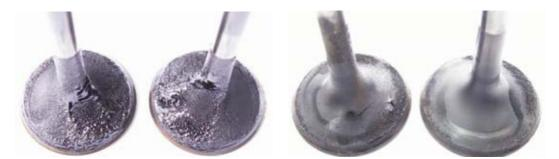
Fig. 5. Intake valve deposits – Mercedes-Benz M111, DOHC, 4 – VPC, electronic Port Fuel Injection [INiG]
