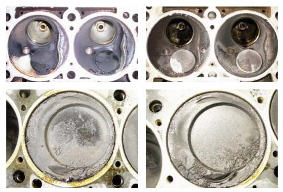
*Fig. 4. Combustion chamber deposits and piston top deposits – Mercedes-Benz M102E, OHC, 2 – VPC, electromechanical Port Fuel Injection [INiG]*
