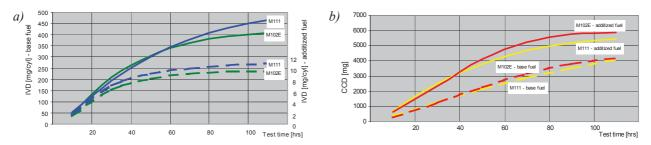
Fig. 8. Comparison of Intake Valve Deposit (a), and Combustion Chamber Deposit (b) for base fuel and additized fuel evaluated in M102E or M111 test engine
