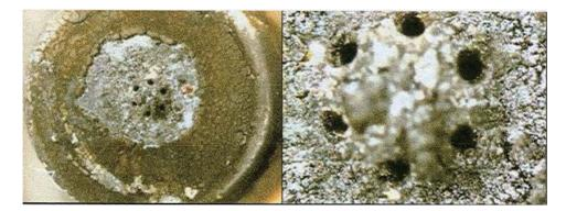
Fig. 7. Fuel deposits on the tip of GDI injector [4]
