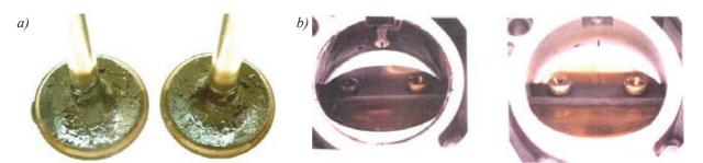
*Fig. 2.* Intake valve deposits (a), and deposits in the area of carburettor throttle (b) – OPEL Kadett, OHV, 2 – VPC, carburettor [INiG]
