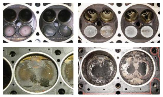
Fig. 6. Combustion chamber deposits and piston top deposits – Mercedes-Benz M111, DOHC, 4 – VPC, electronic Port Fuel Injection [INiG]
