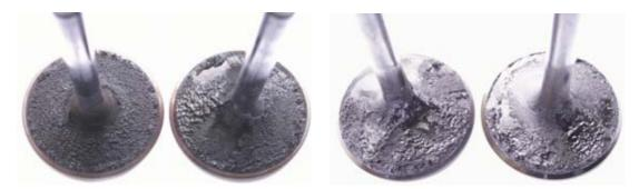
Fig. 3. Intake valve deposits – Mercedes-Benz M102E, OHC, 2 – VPC, electromechanical Port Fuel Injection [INiG]
