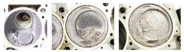
Fig. 9. Examples of deposit flaking in combustion chamber and on the piston top [INiG]
